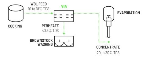
Figure 3. The Via Separations Black Liquor Concentration System removes water directly from weak black liquor.
